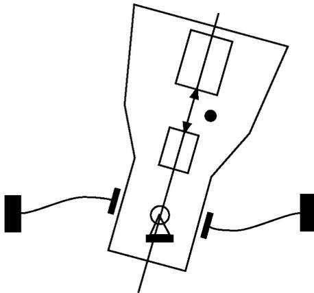
Fig. 4. A multi-rotor gyrostat on an elastic plate.
